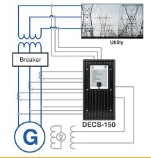
Figure 1 - DECS-150 Connection Diagram for a Typical Application
