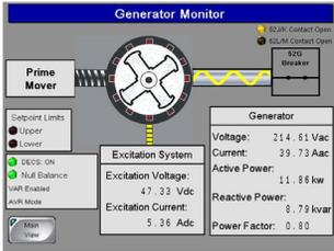
The Generator Monitor screen (left) graphically illustrates excitation system and generator status. Excitation system indicators are provided for ac breaker status, PSS status, field voltage levels, and field current levels. Generator voltage, current, watts, vars, and power factor are also displayed.
