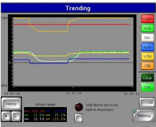
The Trending (left) screens provide access to machine parameters such as generator voltage, apparent power, true power, reactive power, field voltage, and field current. This allows for analysis and review in both graphical and tabular forms. Then, data can be easily exported via USB port in a comma-separated-values (.csv) format.
