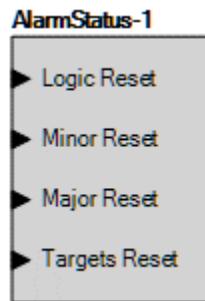
Figure 54-4. Alarm Status Logic Block
