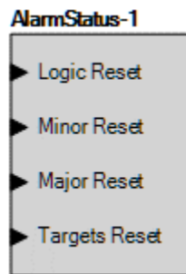
Figure 56-4. Alarm Status Logic Block
