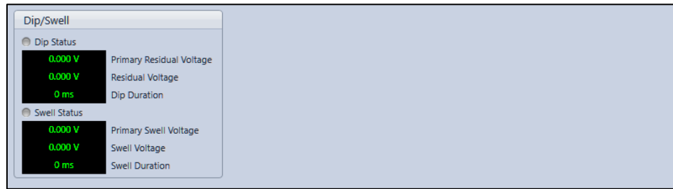
Figure 53-7. Power Quality, Dip/Swell Metering
