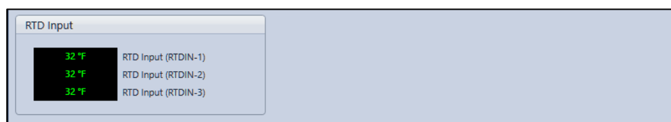
Figure 53-14. RTD Input Metering
